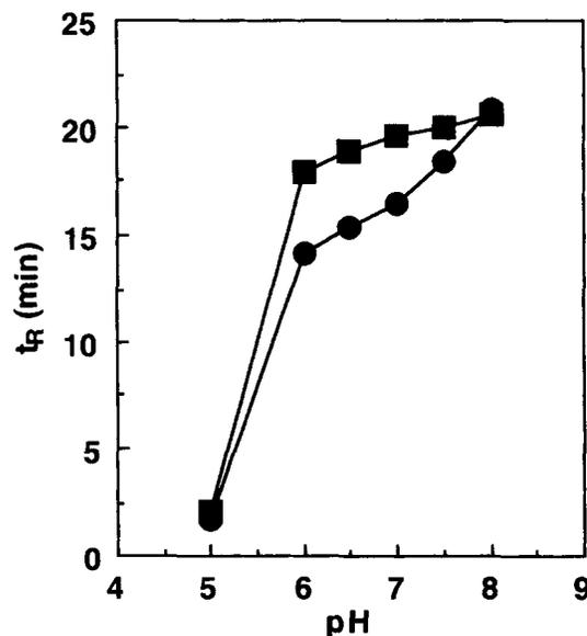
**Figure 4** Effect of eluent pH on retention times of (●) BSA and (■)  $\beta$ -LG on PDAMS-Q(75) column.
