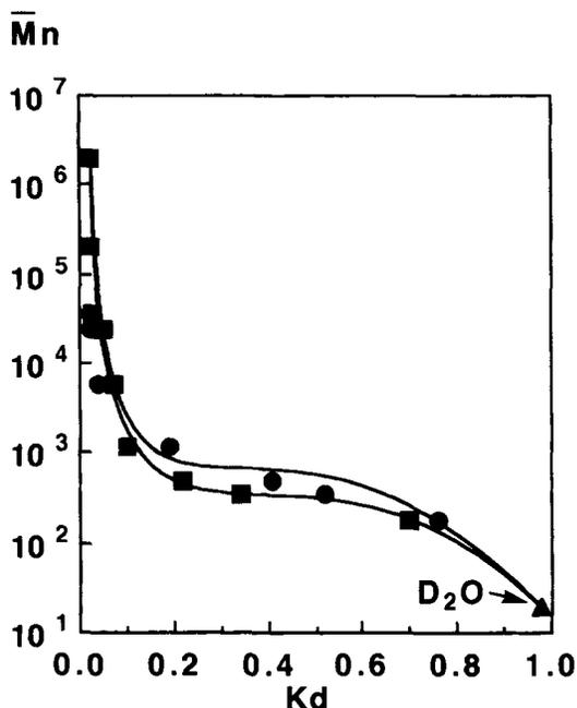
**Figure 2** Calibration curves for (■) PCMS-Q(75) and (●) PDAMS-Q(75) columns using carbohydrates.
