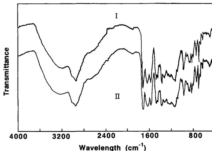
**Figure 1** Typical FTIR spectra of PDAMS-Q(75) (I) and PCMS-Q(75) (II).
