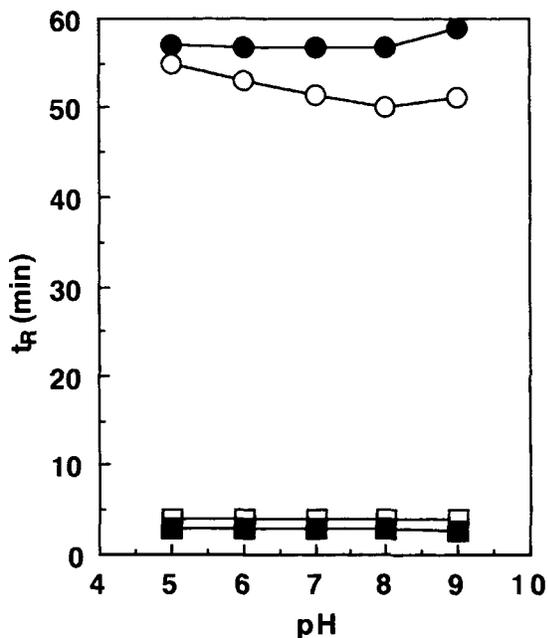
**Figure 3** Relationship between pH of eluent and retention time ( $t_R$ ) on PCMS-Q(75) and PDAMS-Q(75) columns. PCMS-Q column: (□) TMBA; (○) SBS. PDAMS-Q column: (■) TMBA; (●) SBS.
